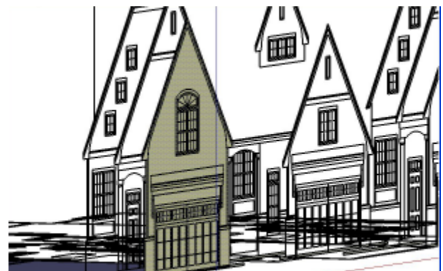
Figure 2c: Elevation is traced to create SketchUp planes, then push/pulled to create 3D massing forms behind elevation. Illus. by Eric Gjerde.
