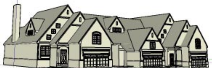
Figure 2c: Elevation is traced to create SketchUp planes, then push/pulled to create 3D massing forms behind elevation. Illus. by Eric Gjerde.
