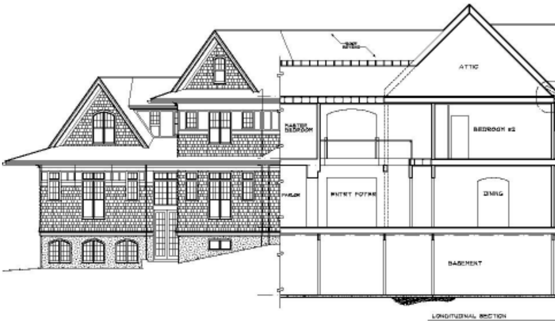
Figure 3: Neil's neat trick to use XClip of elevation to show elevation beyond this section.
