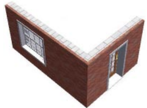
Figure 1: a) 4 line cavity "dumb" walls (upper right) yield barely usable 3D results, but in DataCAD 12 similar b) 4 line "smart walls" (lower pair) deliver 3D renderable results.
